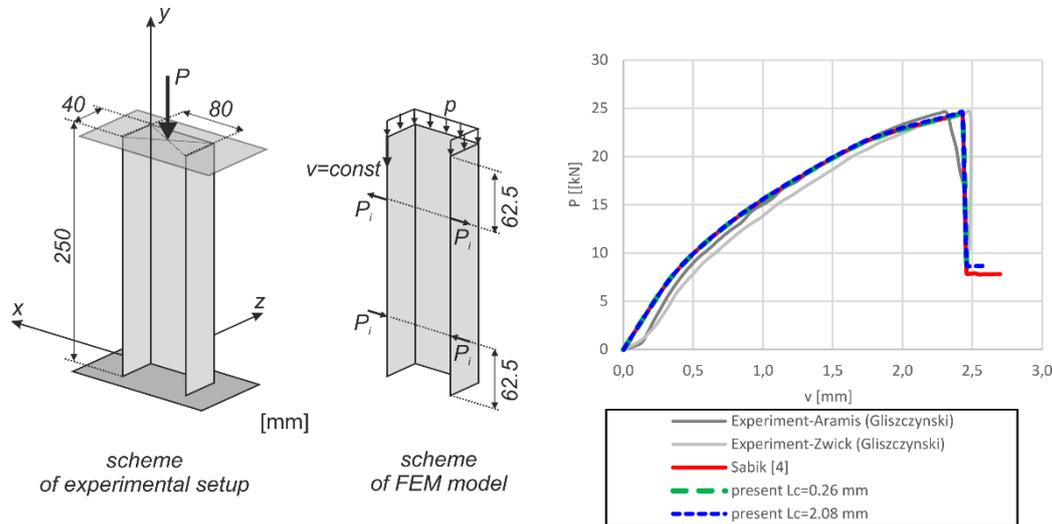
Figure 1: C-shaped column - data and results.
