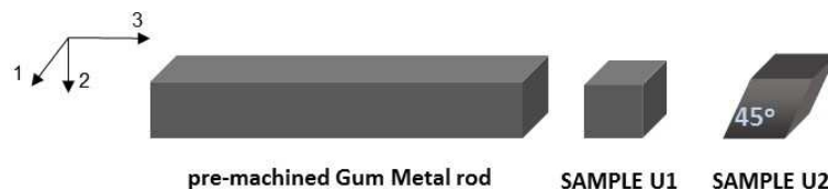
Figure 1: Configuration and orientation of the samples cut out from a Gum Metal rod for ultrasonic test.
