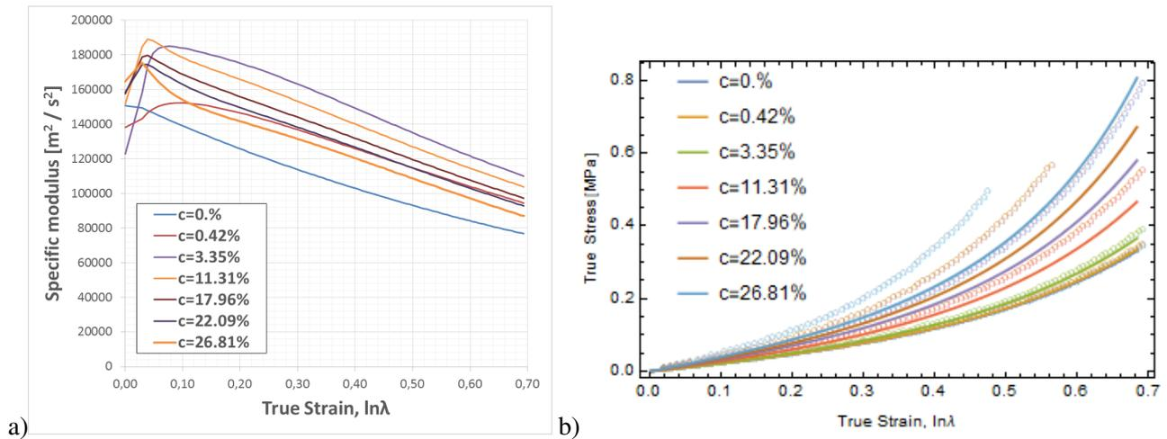
Figure 2: (a) Specific modulus as a function of true strain for steel matrix configuration (only FE analysis) (b) Comparison of true strain-true stress curves obtained by FE analyses (circles) and using micromechanical model (continuous line) for polymer matrix configuration.
