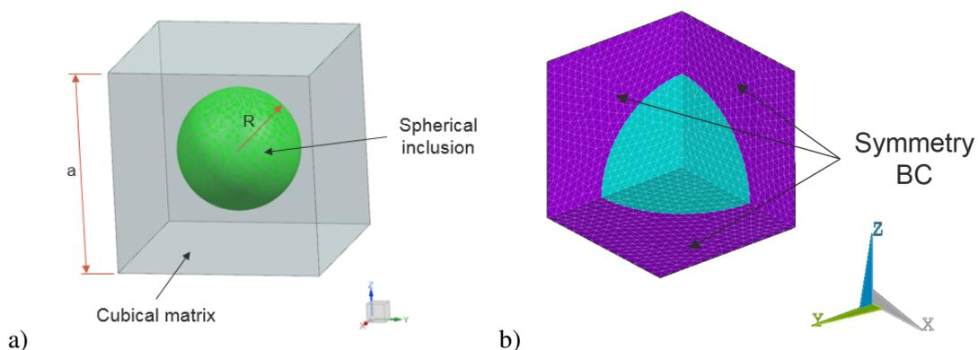
Figure 1: A composite unit cell (a) and its computational model analyzed in ANSYS. (b)
