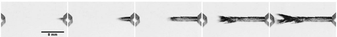
Fig. 1. Crack evolution in V-notched samples with thickness 9.7 mm (recording angle -15^\circ ).
