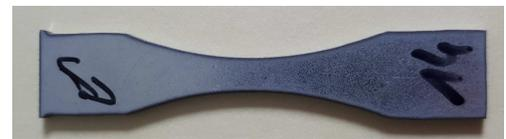
Figure 2: Image of the specimen geometry. The specimens from 1.5 mm DP800 sheets are 50 mm long.
