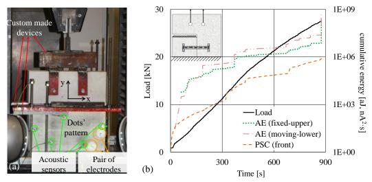
Figure 2: (a) The experimental set-up; (b) Time evolution of the load induced, in juxtaposition to that of the cumulative energy of the Acoustic Emissions and of the Pressure Stimulated Currents.
