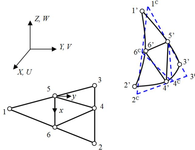
Figure 1. 1-to-6, 1'-to-6' and 1<sup>c</sup>-to-6<sup>c</sup> show the initial, deformed and flat corotational configurations.
