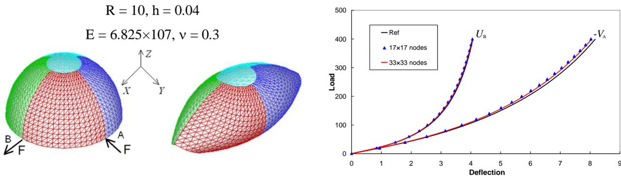
Figure 2. The undeformed and the predicted deformed geometry in a popular elastic shell problem.
