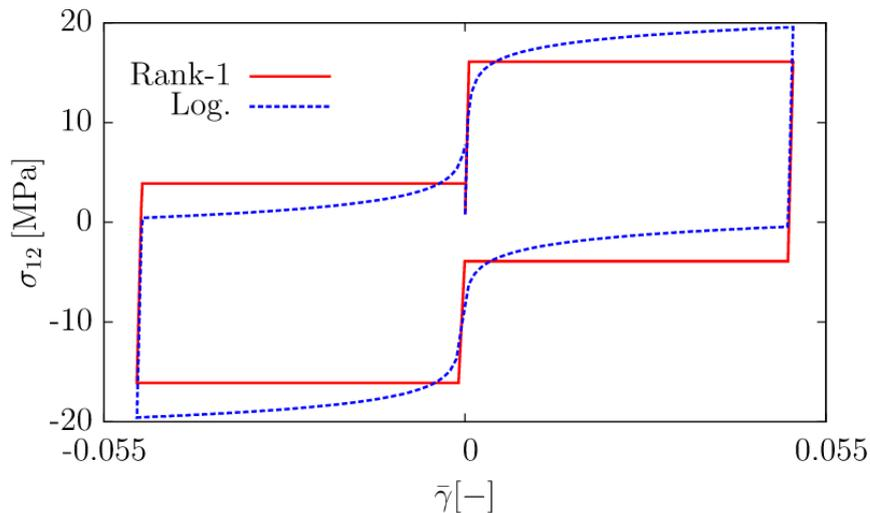
Figure 1: Non-convex cyclic loops in simple shear using two different free energy functions depending on the dislocation density tensor, after [9].
