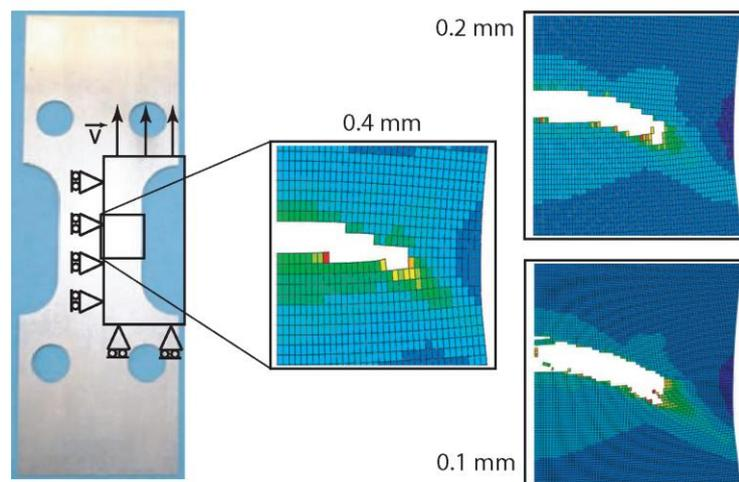
Figure 1: Mesh independent prediction in dynamics using a bounded rate ductile damage model [5]
